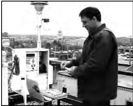
Field technician Fred Currie maintains the PM 2.5 monitors atop the Lincoln Street School in Augusta, Maine.
