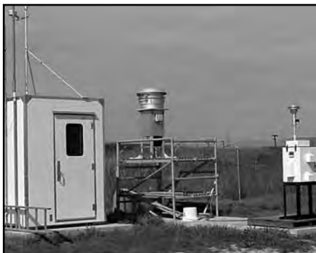
An air quality monitoring station in Woodland, California, that monitors for ozone and fine particulates.
