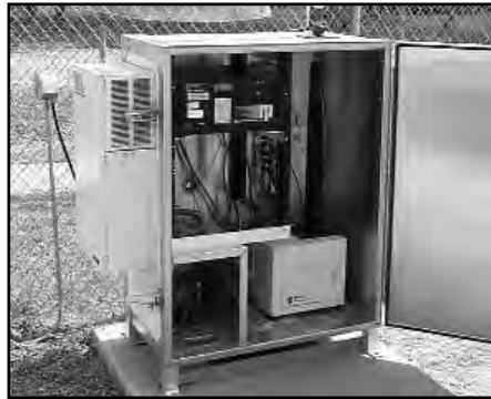
Inside view of a PM 2.5 monitor in Houston, Texas.
