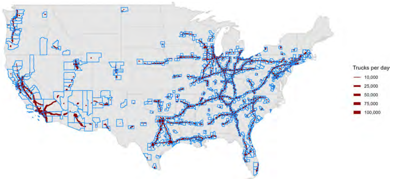
Figure 2: Major Truck Routes and Corresponding Truck Route Counties, 10,000 Trucks per Day Threshold
